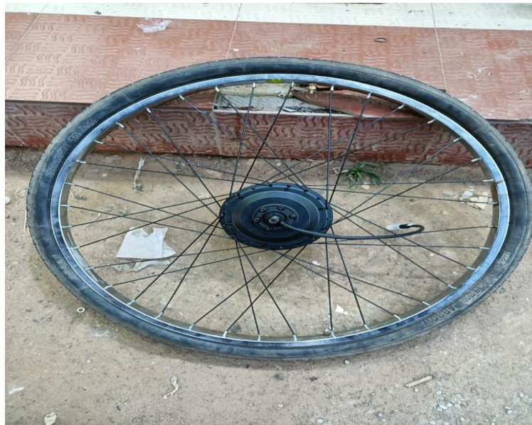
Fig.4.4 Motor fixed in rear wheel rim
