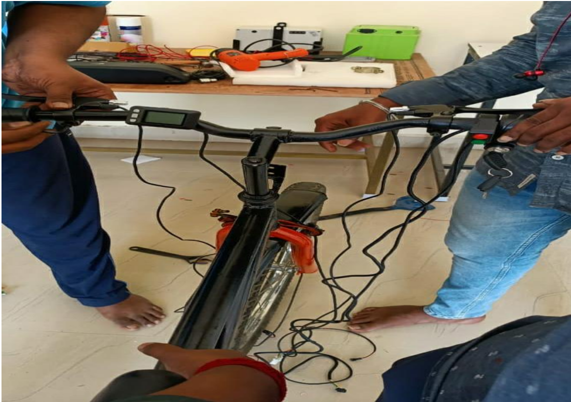
Fig.4.10 Installation of battery, controller and other parts
