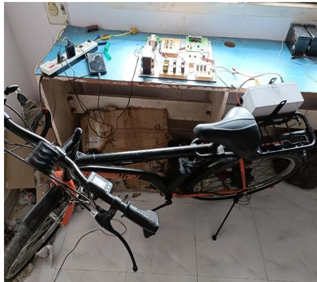
Fig 4.26 E-bicycle charged through pv charging circuit
