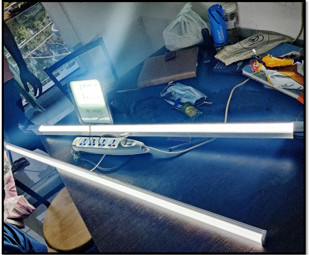
Fig 4.6: Lighting fixtures( 20W batten, 40W batten and 50W Floodlight)
