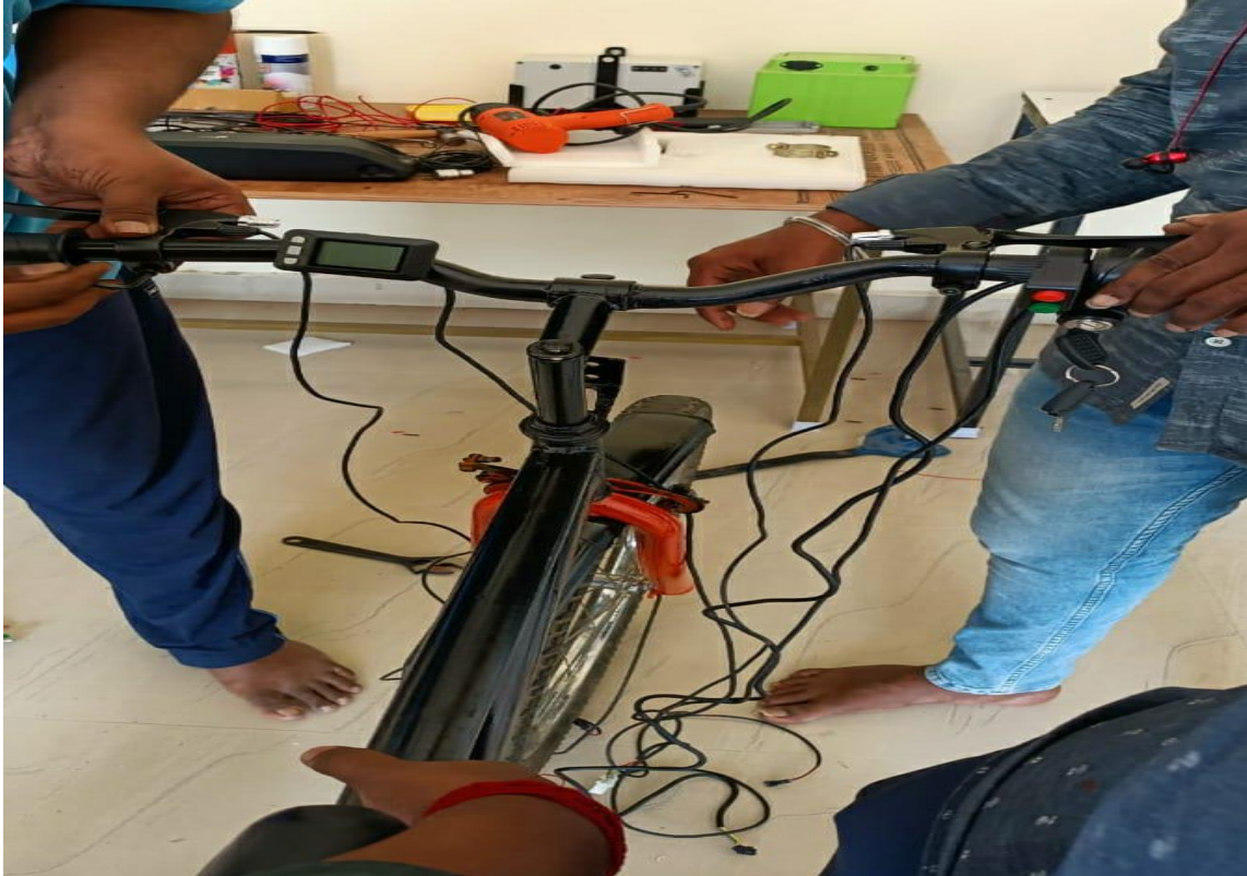
Fig.4.10 Installation of battery, controller and other parts
