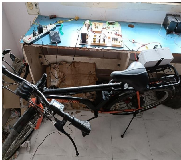
Fig 4.26 E-bicycle charged through pv charging circuit
