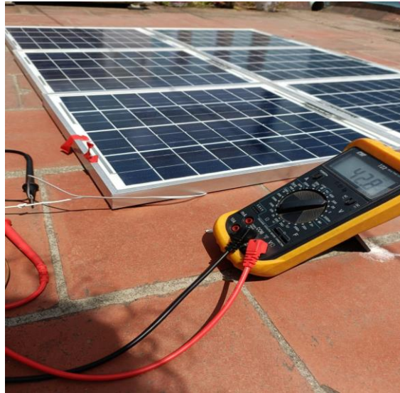
Fig 4.23 Output of panel at maximum radiation
