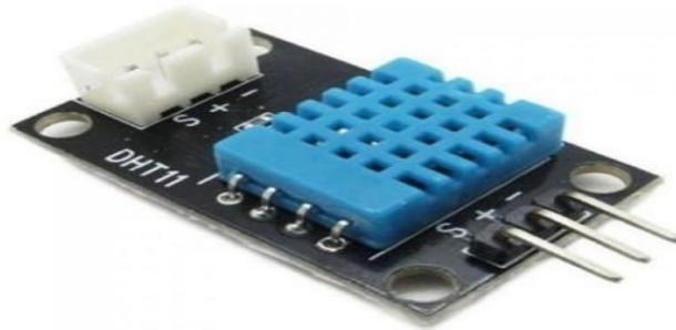
Fig:4.19. Temperature sensor
