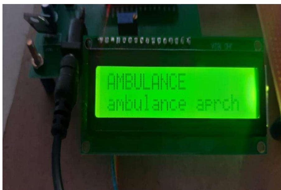
Fig. 6.4: LCD showing ambulance approach
