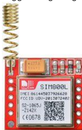
Fig 4.7 : Helical GSM antenna
