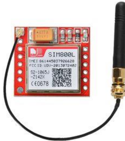
Fig 4.8 : GSM antenna with a U.FL to SMA adapter
