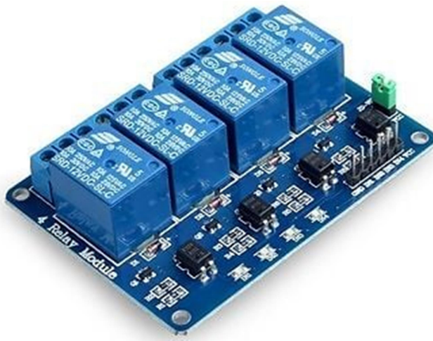
Fig 4.3.1: FOUR CHANNEL RELAY MODULE (Source: [16])
