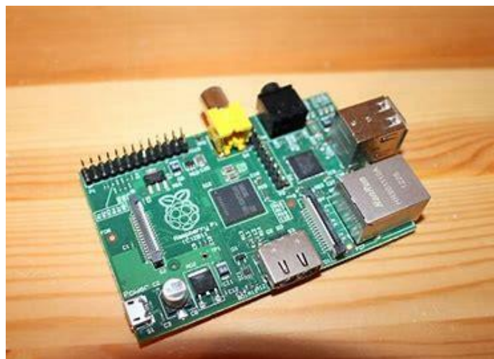
Figure 5-1: Raspberry Pi Model B(Sanders, 2013)
