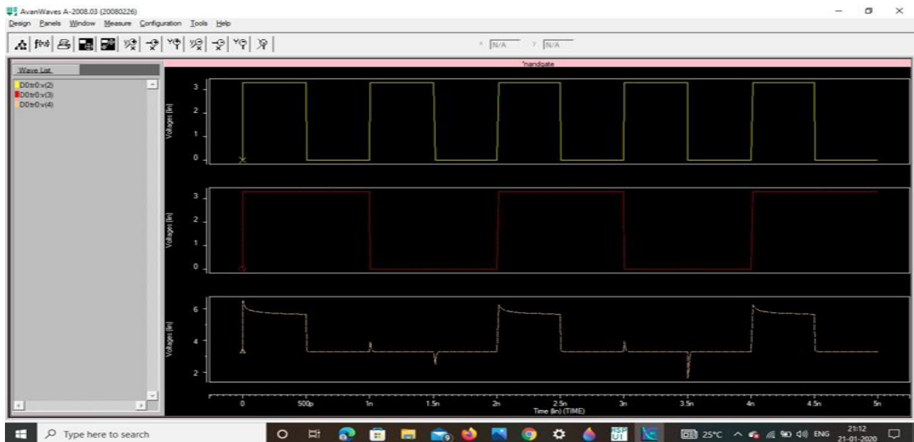
Fig:5.1.2: Simulation Result of NAND GATE
