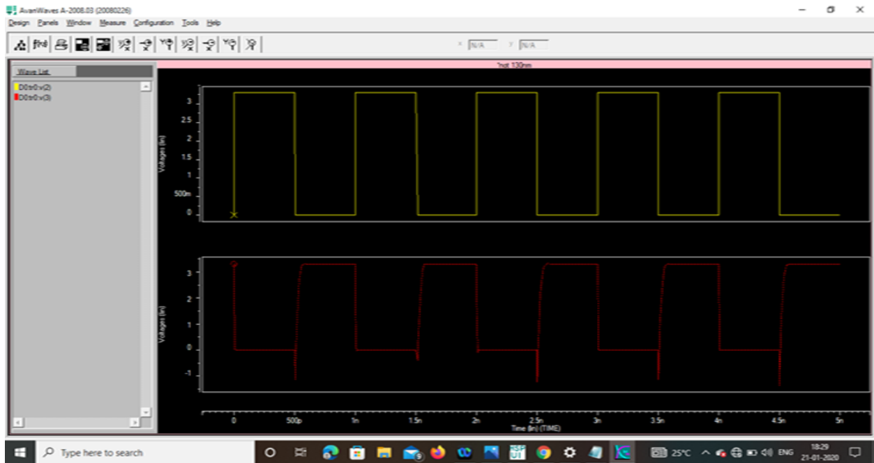
Fig:5.1.1: Simulation Result of NOT GATE
