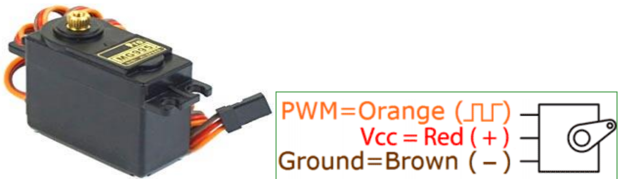
Fig 5.9 Pin Diagram of Servo Motor
