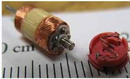
A toy's small DC motor with its commutator
