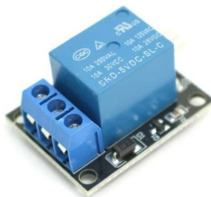
Figure 5.2 Single Channel Relay Module with Opto-Coupler
