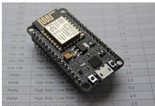
Figure 5.1 NodeMCU ESP8266 Wi-Fi Development Board
