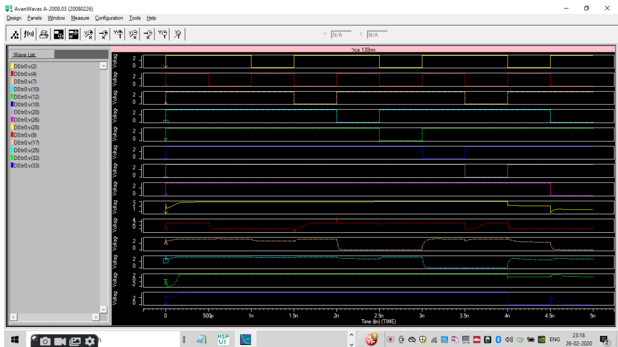
Fig: 5.9: Simulation Result of Proposed 4-Bit RCA
