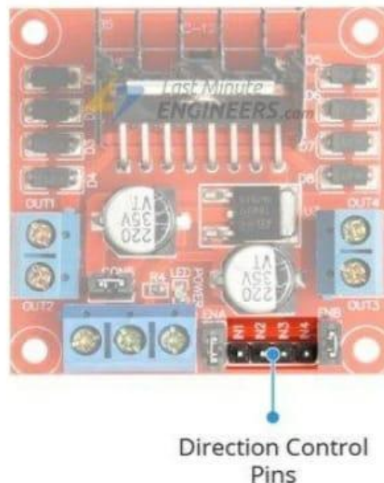
FIG. 4.23: CONTROL PINS OF L298N CHIP
