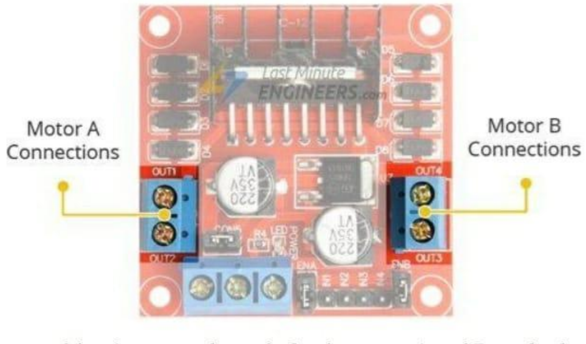
Fig. 4.22: OUTPUT PINS OF L298N CHIP
