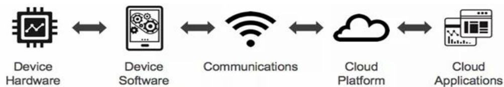
Fig. 4.6: The IoT Technology Stack
