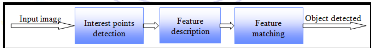
Fig 4.1 Flowchart of SURF algorithm
