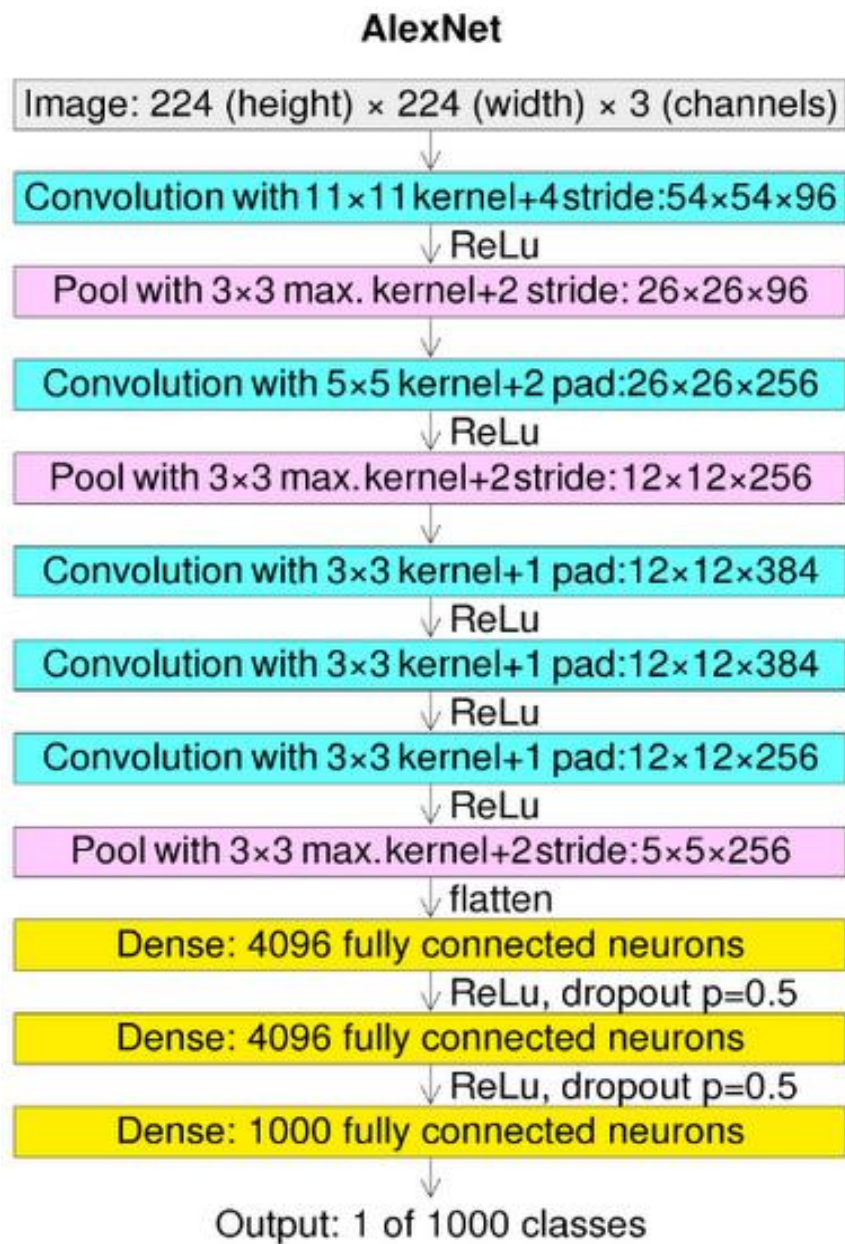
Fig 13: Architecture of AlexNet
