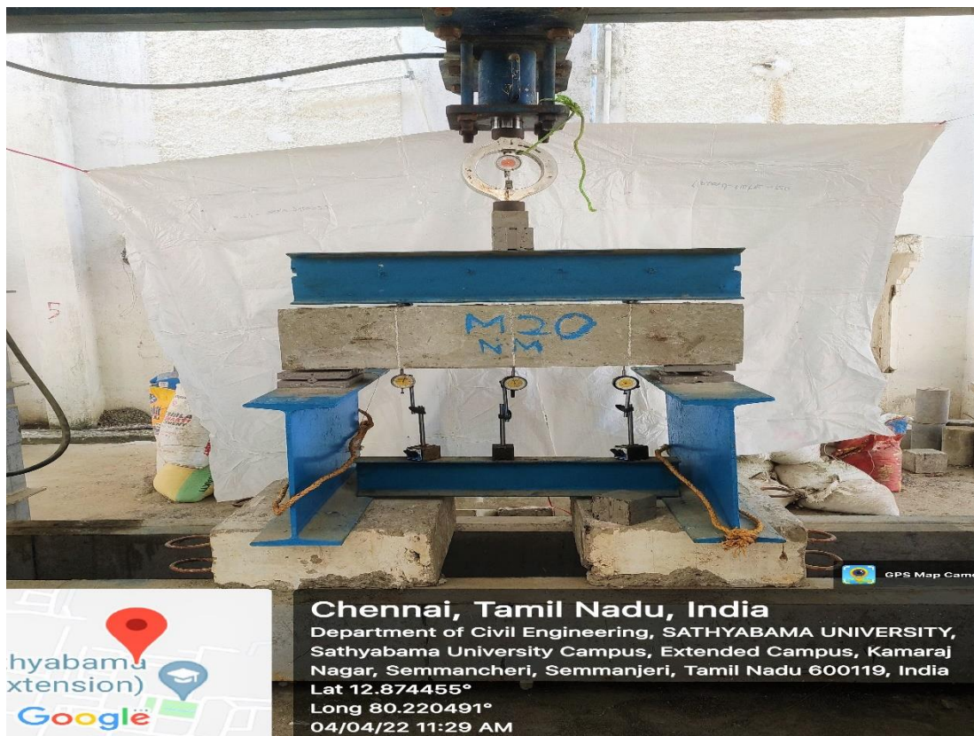
Fig: 4.8: Experimental Set up for M20 Grade Conventional Beam
