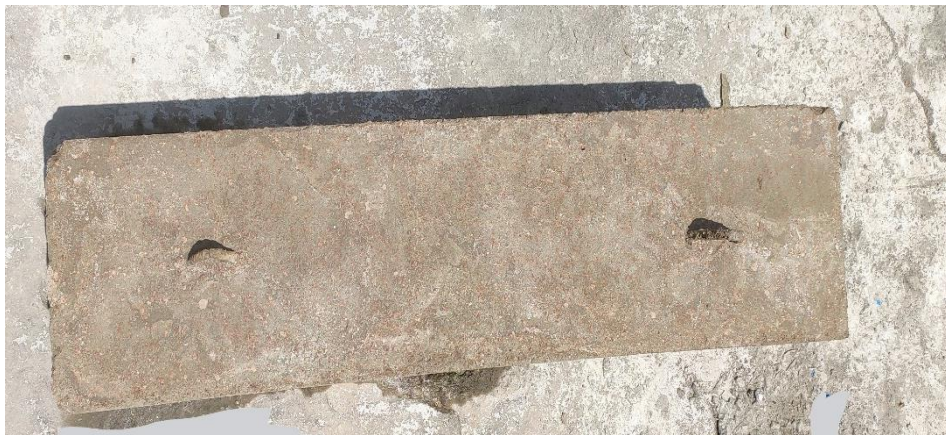
Fig: 4.5: Demoulded RC Beam
