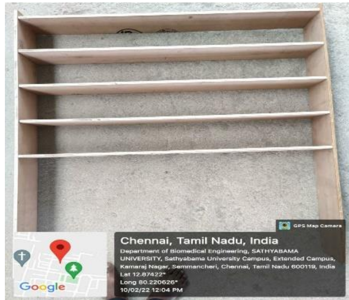
Fig:4.3 Frame for RCC beam
