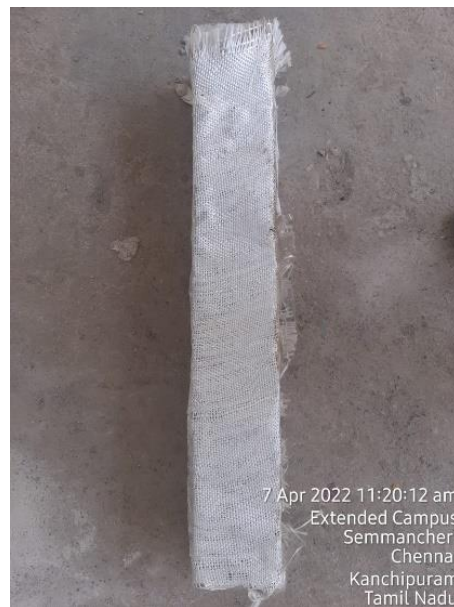
Fig:5.6 Beam wrapped with glass fiber
