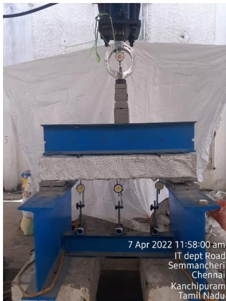
Fig:5.5 Beam wrapped with glass
