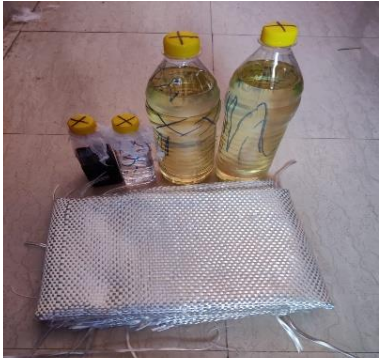
Fig:4.4 Polyester and reinforced glass fiber
