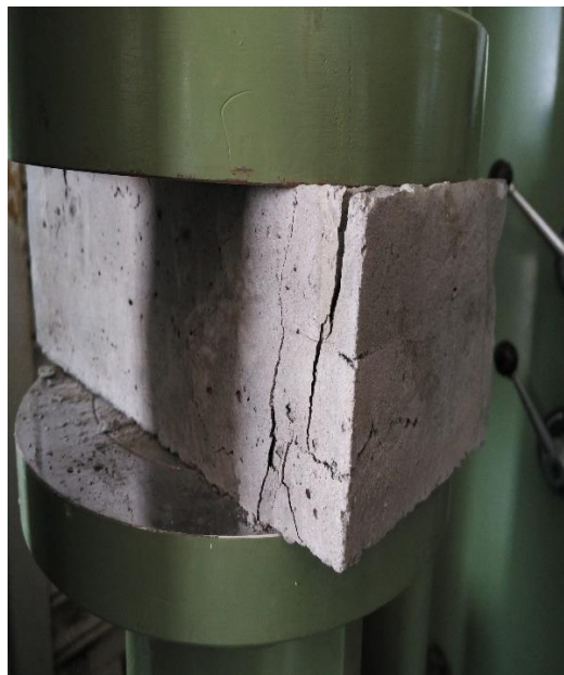
Fig 4.4: Compression Test on Block
