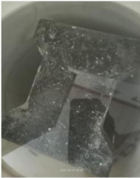
Fig 4.2: Water Absorption Test of Concrete blocks that interlock
