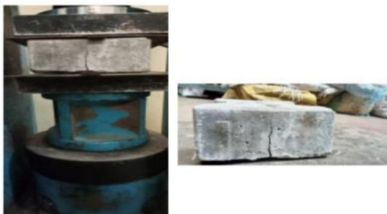
Fig 4.4: Tensile splitting test on interlocking concrete blocks
