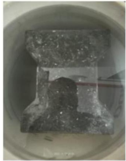
Fig 4.2: Water Absorption Test of Concrete blocks that interlock
