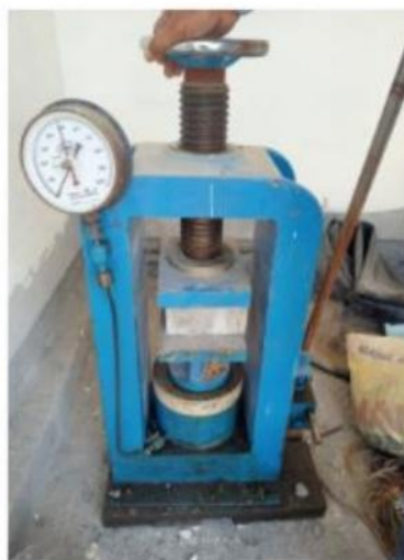
Fig 4.3: Compression test on interlocking concrete blocks
