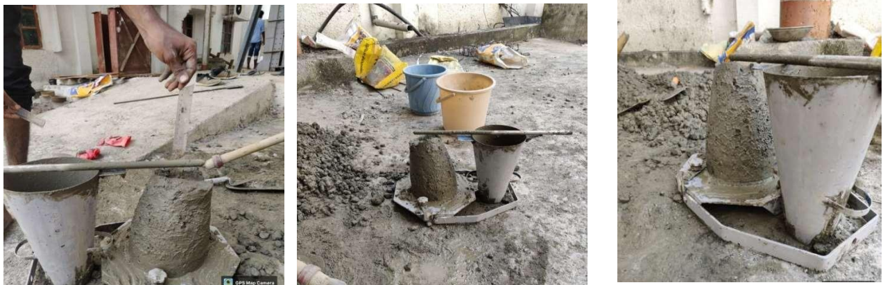
Fig 5.7 Fresh concrete test on nominal, Mix1and Mix2 respectively
