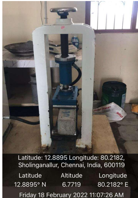
Fig.5.12 Picture of flexural test on concrete
