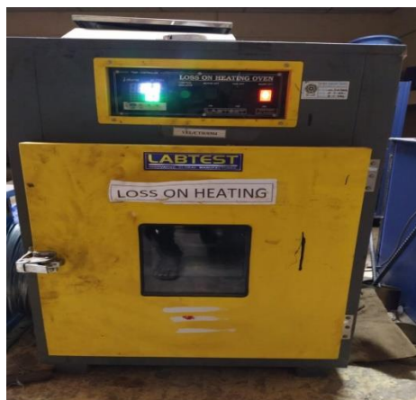
Fig: 5.4: Loss on heating test machine
