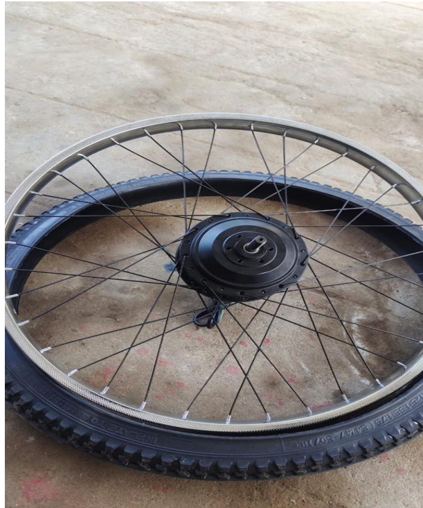
Fig 5.4 36v 350w BLDC hub motor
