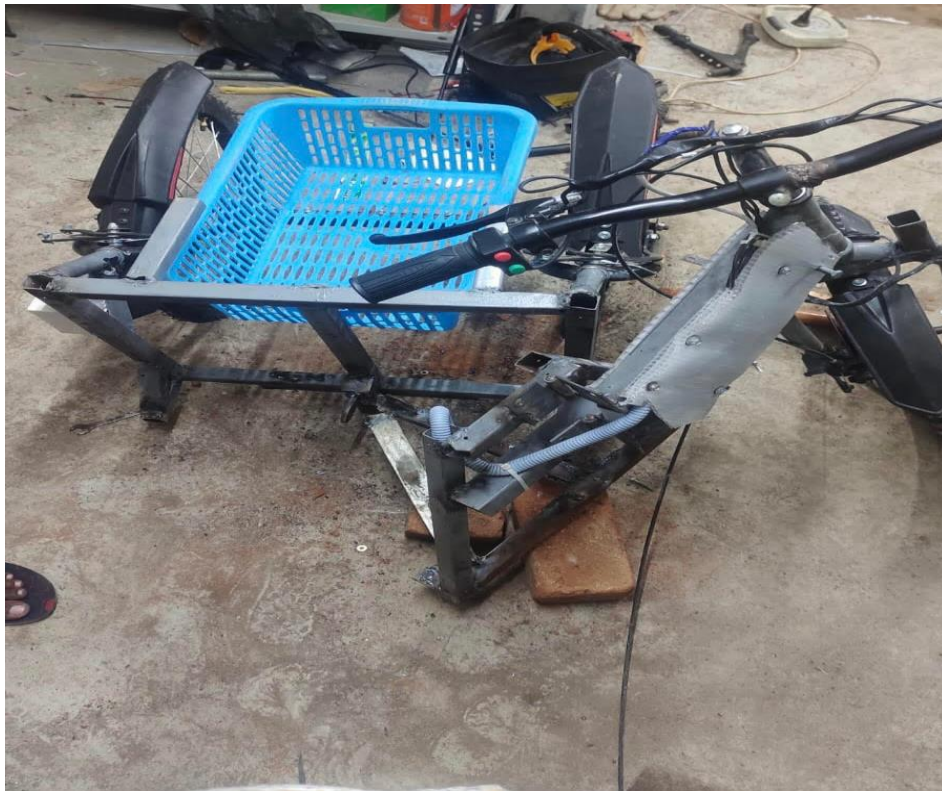
Fig 5.3 Final Folding Of Three wheeler
