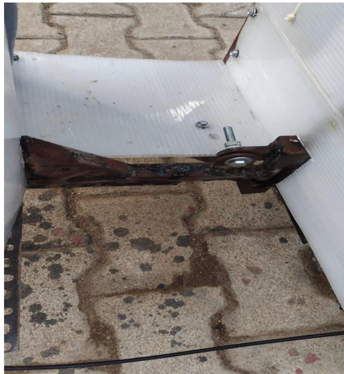
Fig 5.9 Hinge at the mid section of three wheeler
