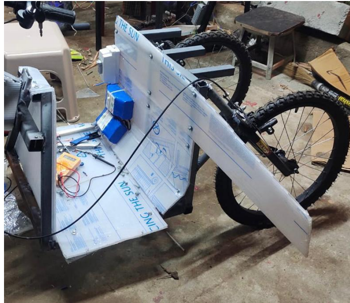
Fig 5.10 Initial assembly of components of three wheeler.
