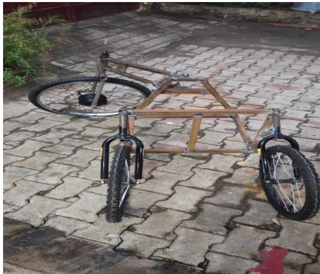
Fig 5.2 Initial Folding Of Three wheeler
