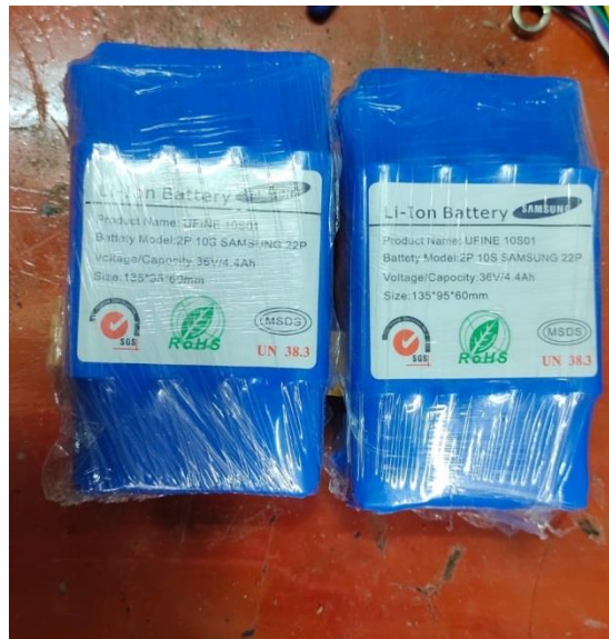
Fig 5.5 36v Li-ion battery
