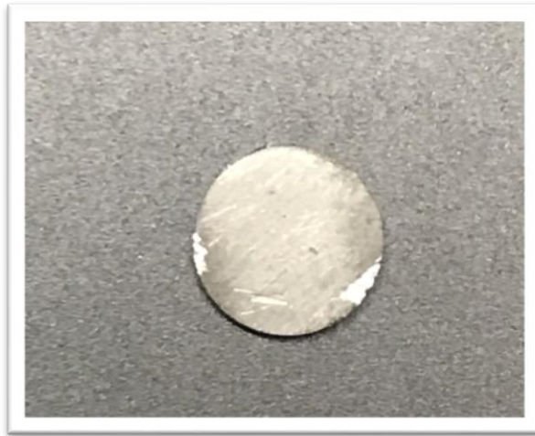
Fig 4.3 Sample size 2mm thickness 8mm diameter
