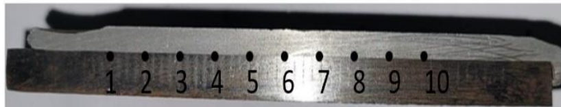
Fig 5.1. Half-cut material for Vertical hardness test
