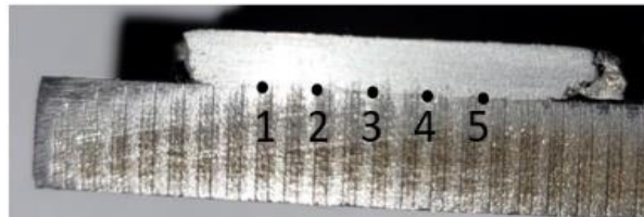
Fig 5.2. Traverse cut material for hardness test
