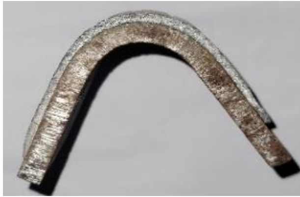
Fig 5.5. Face bend sample material
