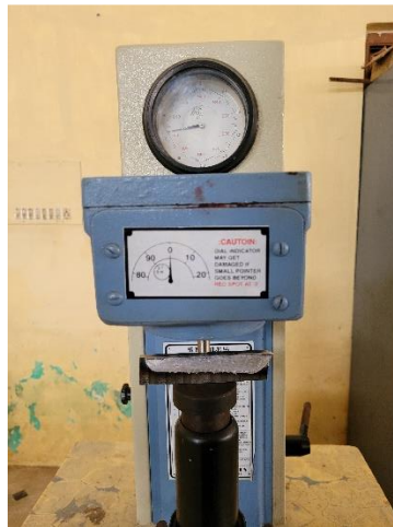
Fig 5.3. Rockwell microhardness testing machine.
