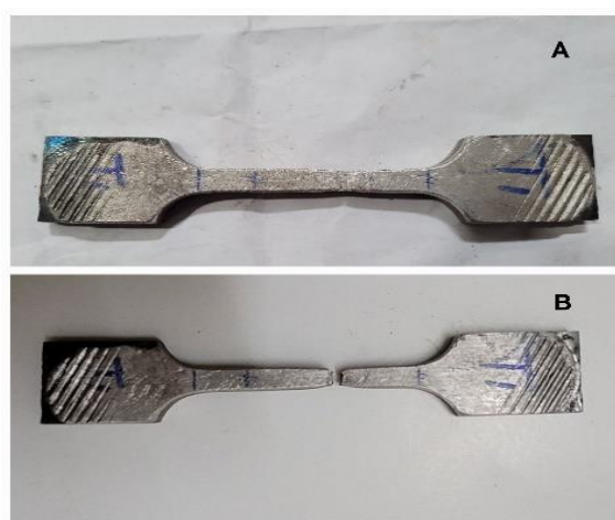
Fig 5.6. A – Before tensile test B – After tensile test
