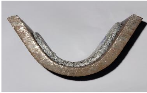
Fig 5.4. Root bend sample material
