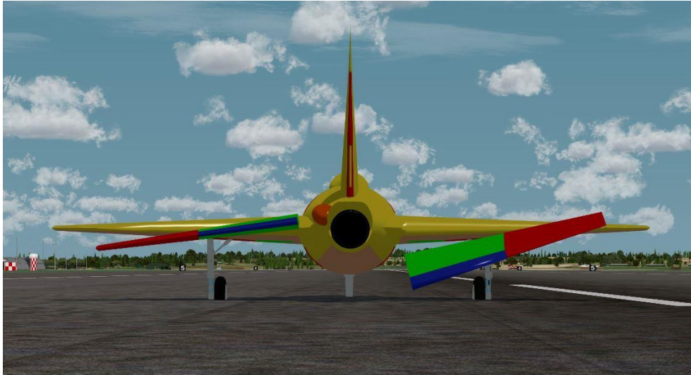
fig.6: Elevons function during pitch down movement
