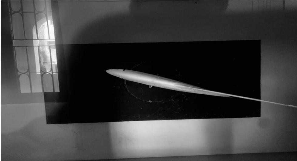
fig.34: Experimentation of 3d model in a wind turbine with varying angles of attack
