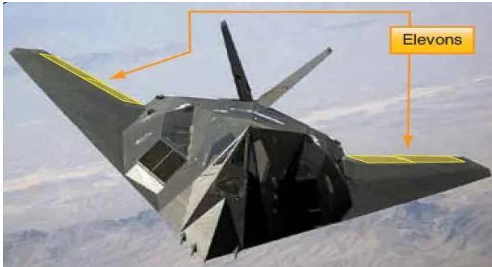
Fig.3: Representation of elevons in Northrop series aircraft
