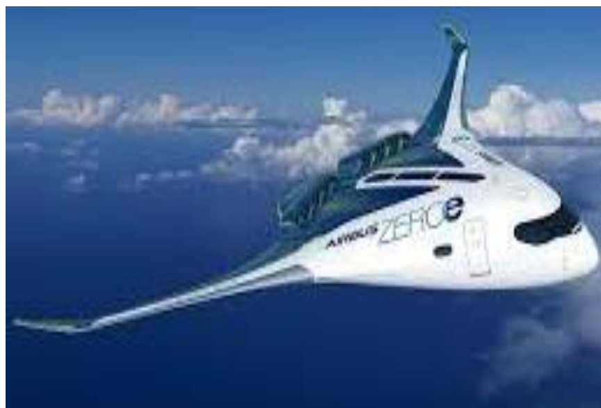
Fig: 1.1 Blended Wing Body
