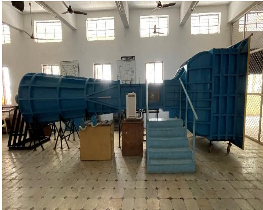
Fig: 7.1 Subsonic Wind Tunnel
