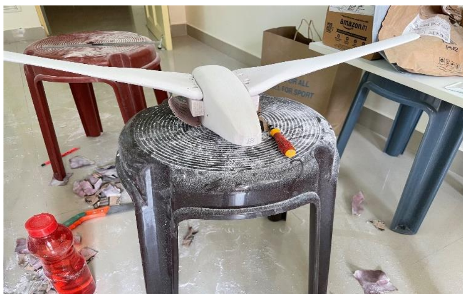
Fig: 6.3 Smooth body after Sanding
