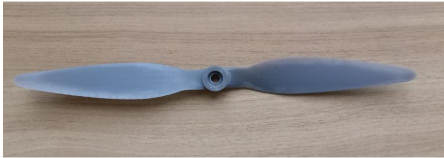
Fig 4.28 Second Version of Propeller after printing
