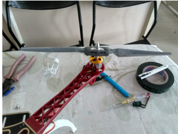
Fig 4.39 First Version of custom Propeller
