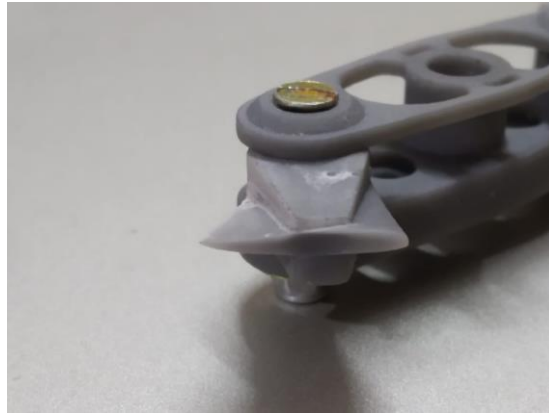
Fig 4.41 Point of Failure of first version
