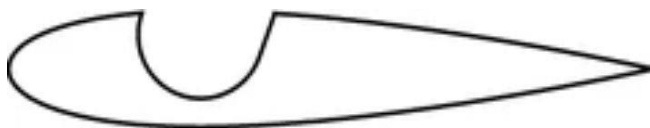
Fig.11: Semi circle cavity slot in airfoil
