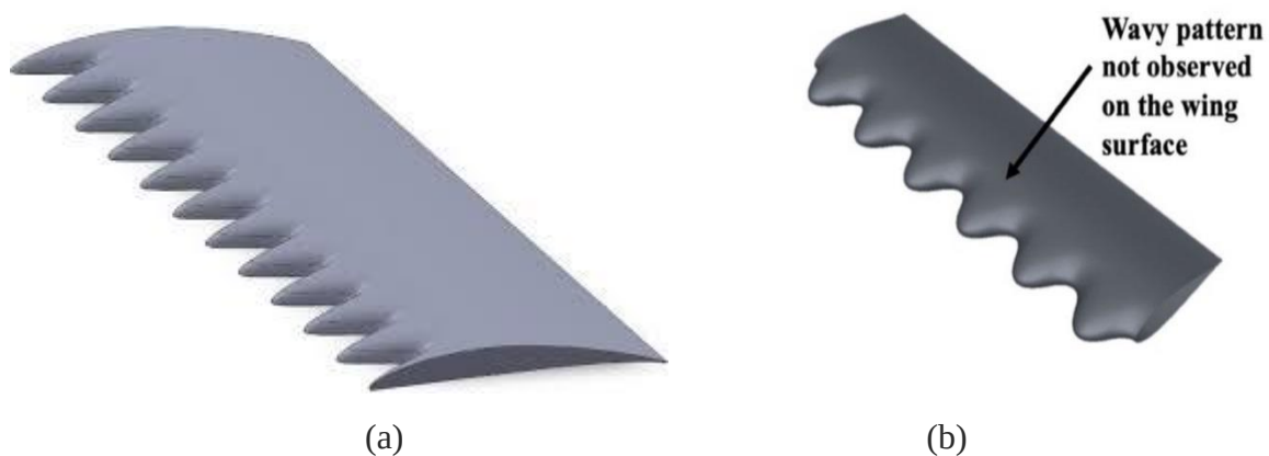
Fig.13: (a) Serration in leading edge of airfoil
