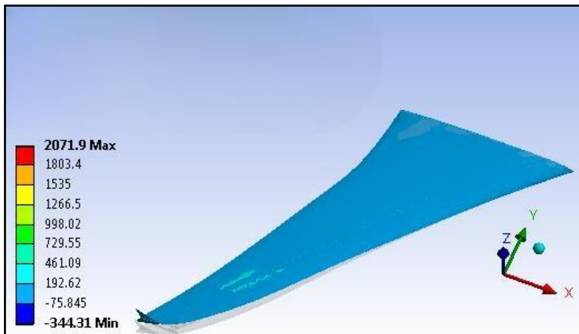
Figure 5.34: Max Principal Stress Results (Model 1)
