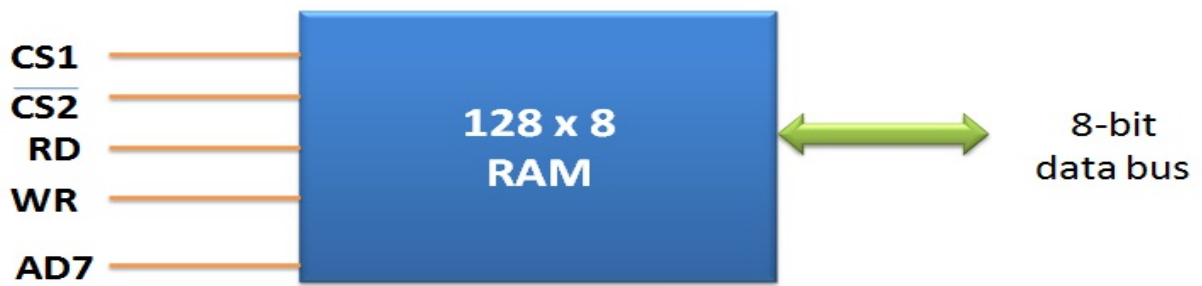
Block Diagram Representing 128 x 8 RAM (Random Access Memory)
