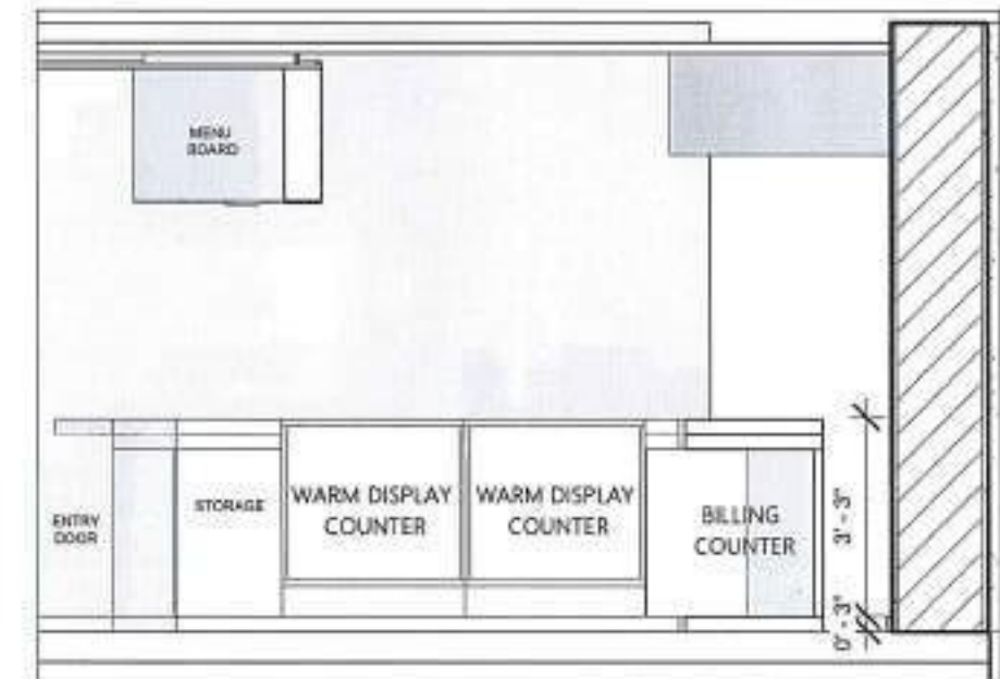
③ SECTION B (WARM COUNTER FACING) 1 : 40
