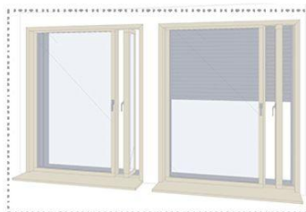
Windows allow the autonomy of patients to control ventilation ( safe dimension of 15cm of free opening ) and rolling shutter.
