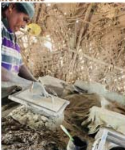
Step 6: levelled and compress the wet mixture to avoid uneven surface.
