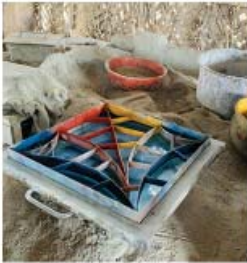
Step 1: Placing the mould over the glass which is fitted into the frame
