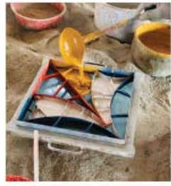
Step 2: Pouring the decided pigment mixture into the mould.
