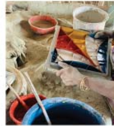
Step 3: Spreading pigment mixture equally
