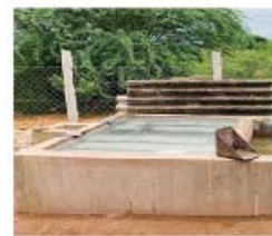
Step 9: After the tile got dried, they soak the tile in water for 15 days
