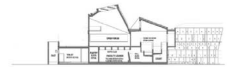
Cross section through the open forum and ramp of the academic block
