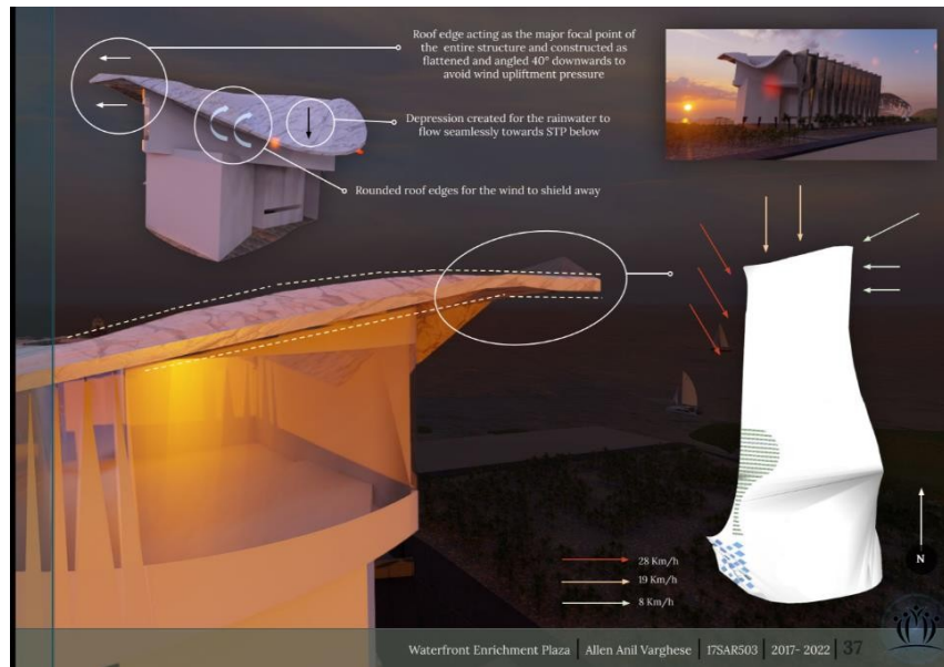
Plate3.16 -Roofstructuredetails
