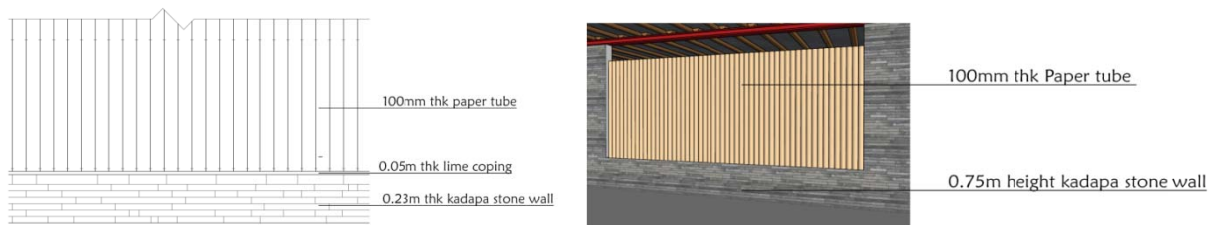
Fig 5.10(a),(b): Construction of wall system
