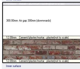
Fig 4.16: AAC block with ACP cladding
