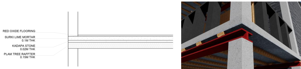
Fig 5.10 : Construction of roof system
