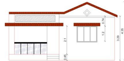
fig 5.10 Elevation of new Kota house
