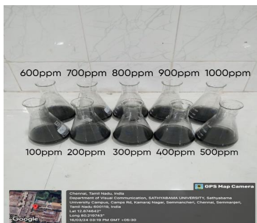
Figure:5.11: Ofloxacin Concentration on adsorption using AC-MgO- \text{Fe}_3\text{O}_4
