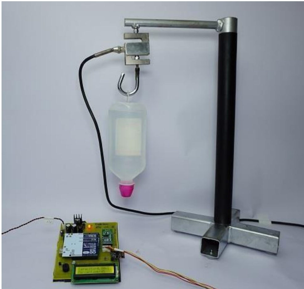
Fig .1.4 Drip Control System
