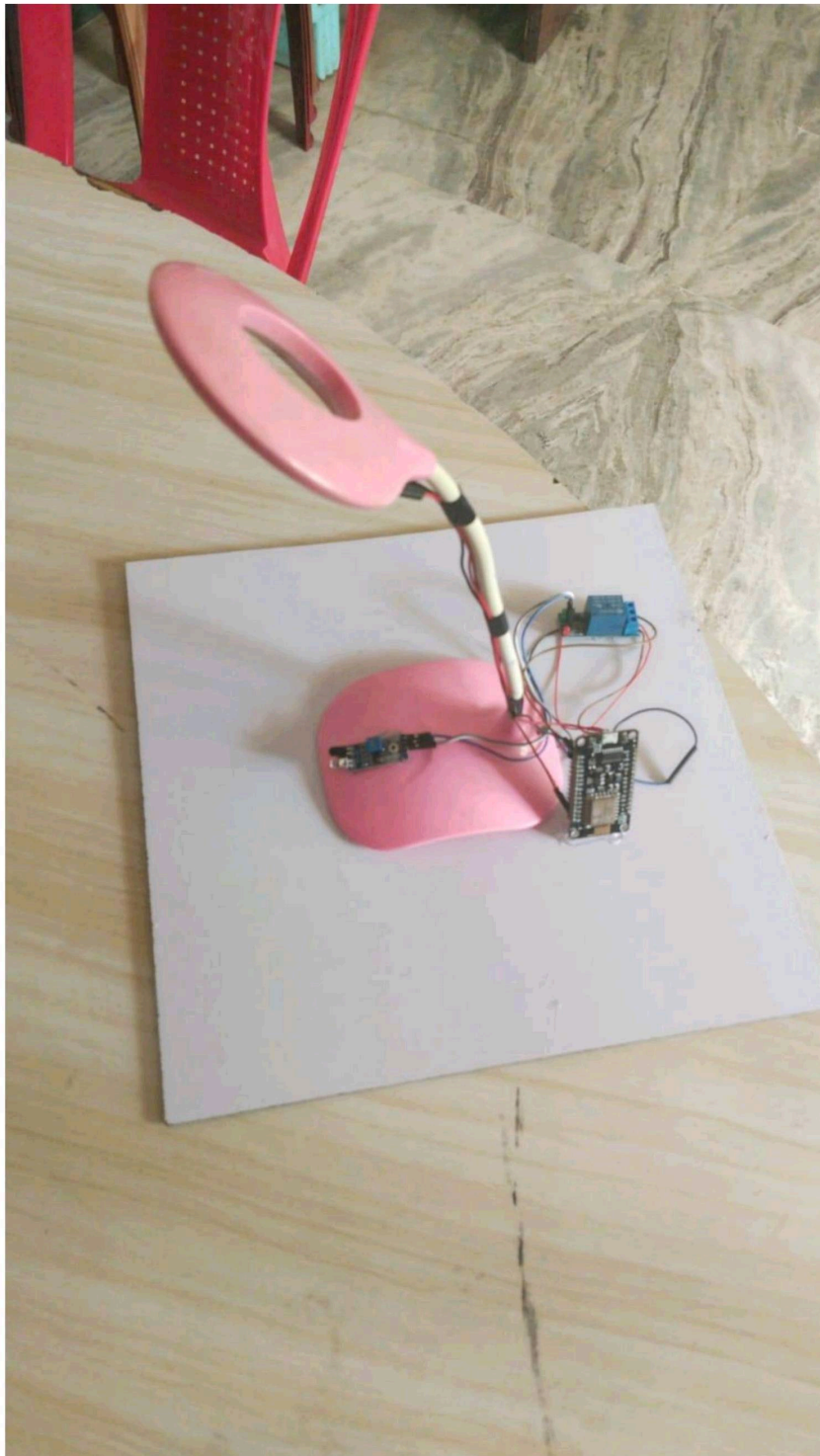
Fig:6.1: Right-side view(LDR,PIR connected to light through relay and arduino uno)
