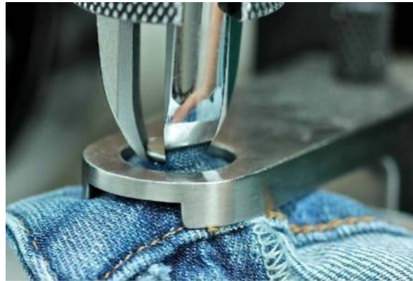
Figure 34 Buttoned Pulling Test
