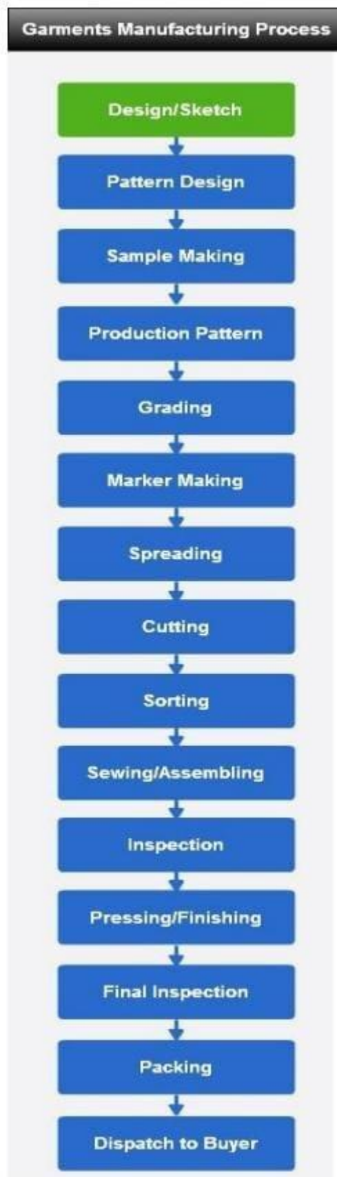
Figure:6 Garments manufacturing process
