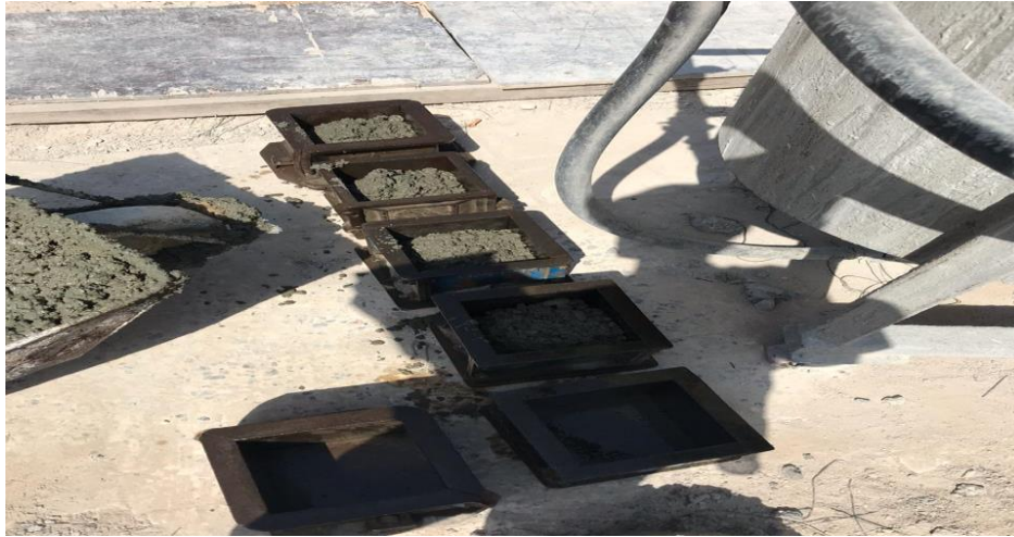
Fig 4.6: Casting of Specimen
